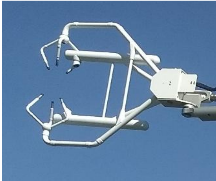
Fig. 3. 5 The Eddy covariance sensor installed at Nagani AWS station
