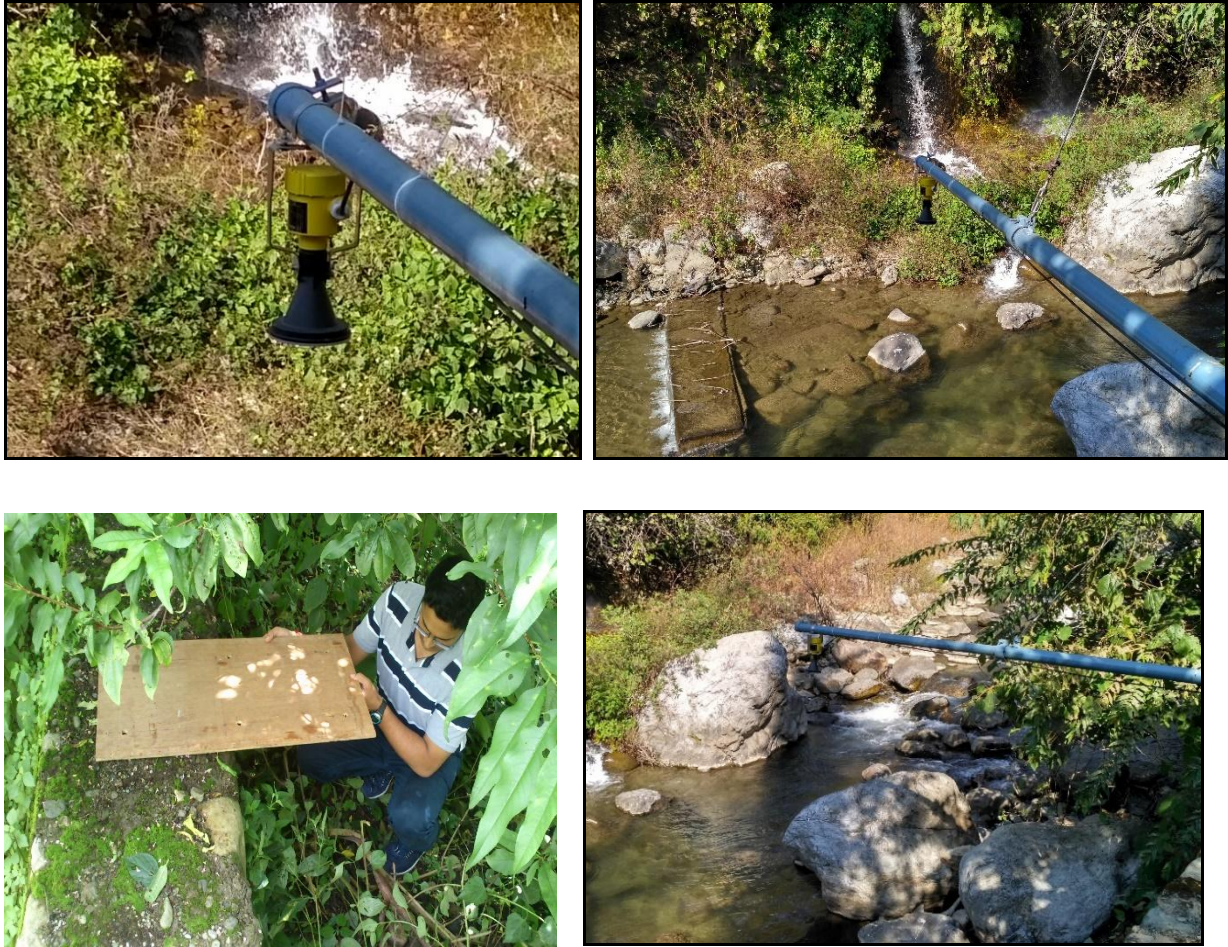
Fig. 3. 3 The digital water level recorder (DWLR) installed on the outlet of Henval stream at Jijali-Devnagar
